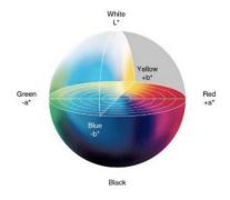
The CIE-Lab color difference equation calculates coordinates to locate a point in the in the three-dimensional sphere model. The coordinates are for the L\*, a\* and b\* axis. L\* is a measure of lightness to darkness. a\* is the red to green axis and b\* is yellow to blue. Color differences are calculated from these coordinates and represent the distance between the target and trial along each axis.
